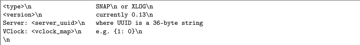
After the file header come the data tuples. Tuples begin with a row marker 0xd5ba0bab and the last tuple may be followed by an EOF marker 0xd510aded. Thus, between the file header and the EOF marker, there may be data tuples that have this form:
