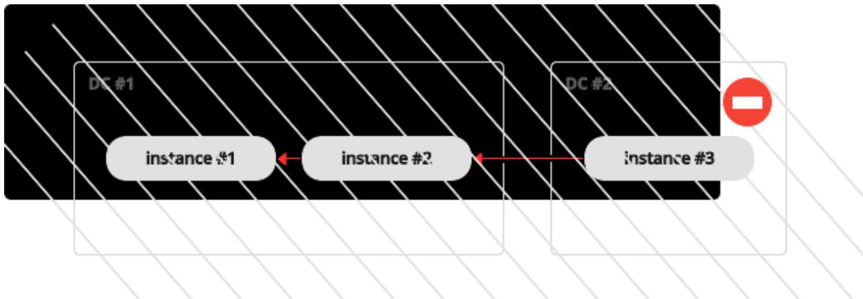
The problem with a cascading replica set is that some instances have no connection to other instances and may not receive changes from them. One essential change that must be propagated across all instances in a replica set is an entry in `box.space._cluster` system space with replica set UUID. Without knowing a replica set UUID, a master refuses to accept connections from such instances when replication topology changes. Here is how this can happen:
