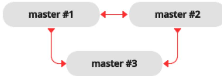
You then can decide where to locate instances of the mesh – within the same data center, or spread across a few data centers. Tarantool will automatically ensure that each row is applied only once on each instance. To remove a degraded instance from a mesh, simply change `replication` configuration parameter.
