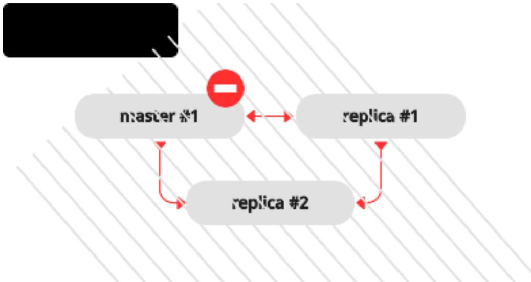
In a master-replica set, if a master disappears, error messages appear on the replicas stating that the connection is lost:
