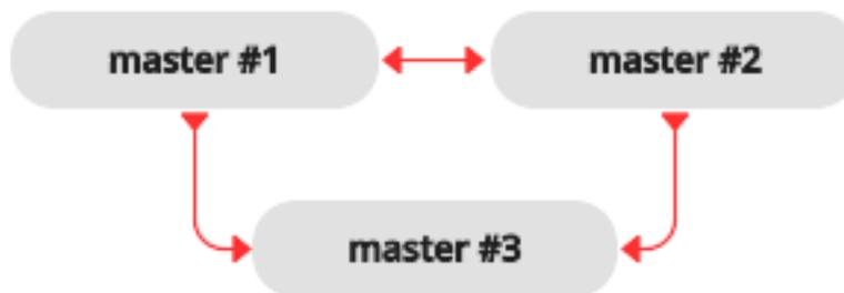
The failover benefit in this case is still present, and the load-balancing benefit is enhanced, because any instance can handle both read and write requests. Meanwhile, for multi-master configurations, it is
