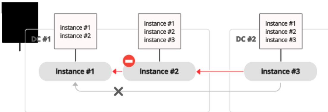
Now instance #2 is faulty. Instance #3 tries connecting to instance #1 as its new master, but the master refuses the connection since it has no entry for instance #3.
